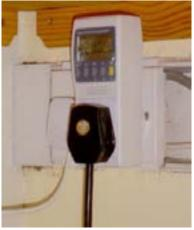
It is also possible to undertake such measurements on three phase supplies using a three phase electrical data logger. Again this uses current transformers to measure current, and is usually connected to the electrical supply directly to sense voltage. This connection to sense current and voltage on all three phases must be undertaken by a competent person.
