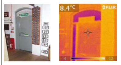
Temperatures in thermal infrared images are frequently represented in artificially generated colours to enhance the visual contrast arising from small temperature differences, but as an alternative, most cameras can be set to display a black and white image where the hotter objects are shown as brighter white.
