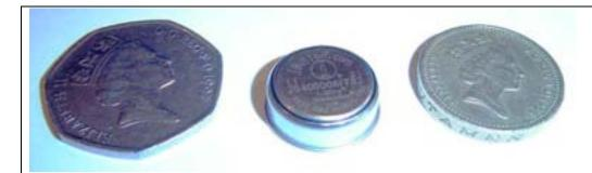
As an example, the DS1921 Thermochon stores 2048 temperatures, and can be programmed to record temperature readings at any interval between 1 and 255 minutes. If the device is set to record temperatures every 10 minutes, it can record temperatures for a little over two weeks, with good enough resolution to allow the details of any particular day to be explored. The devices cover an operating temperature range of -50°C to +100°C, and can be obtained for £5 to  $\pm$ 10 each.
