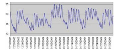
Note that while the heating was correctly turned off on days when the office was closed, it was routinely overheated on many working days. The following graph uses an extract of the same data to show half hourly temperatures for the 8<sup>th</sup> of January only.
